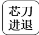
Core Knife In/Out Button: In manual or test mode, pressing the button once retracts the core knife, and pressing it again advances it.
